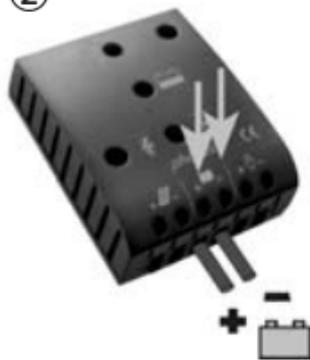
Connect the wires leading to the battery with correct polarity. To avoid any voltage on the wires, first connect the controller, then the battery. Keep in mind the recommended wire length (min. 30 to max approx. 100 cm) and the wire size:
