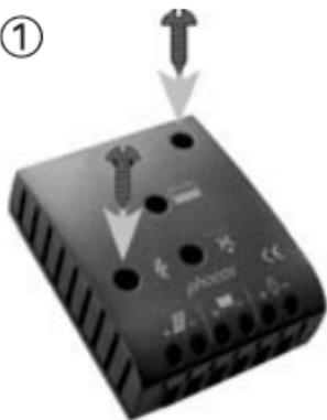
When mounting the controller with screws, make sure to use screws that suit the attachment material (use screws with 4 mm shaft and max. 8 mm head diameter, no counter sink). Keep in mind that the screws also have to carry the force applied by the wiring. Make sure that the ventilator slits on the sides are unobstructed.
