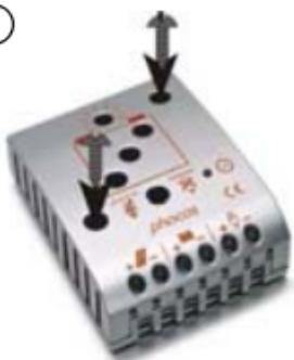
Mount the controller to the wall with screws that fit to the wall material. Use screws with 4 mm shaft and max. 8 mm head diameter, no counter sunk. Mind that the screws have to carry also the force applied by the wiring. Make sure that the ventilator slits on the sides are unobstructed.
