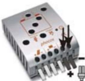
Connect the wires leading to the loads with correct polarity. To avoid any voltage on the wires, first connect the wire to the load, then to the controller. Mind the recommended wire size:
