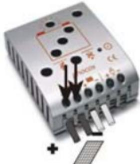
Connect the wires leading to the solar array with correct polarity. To avoid any voltage on the wires, first connect the controller, then the solar array. Mind the recommended wire size:
